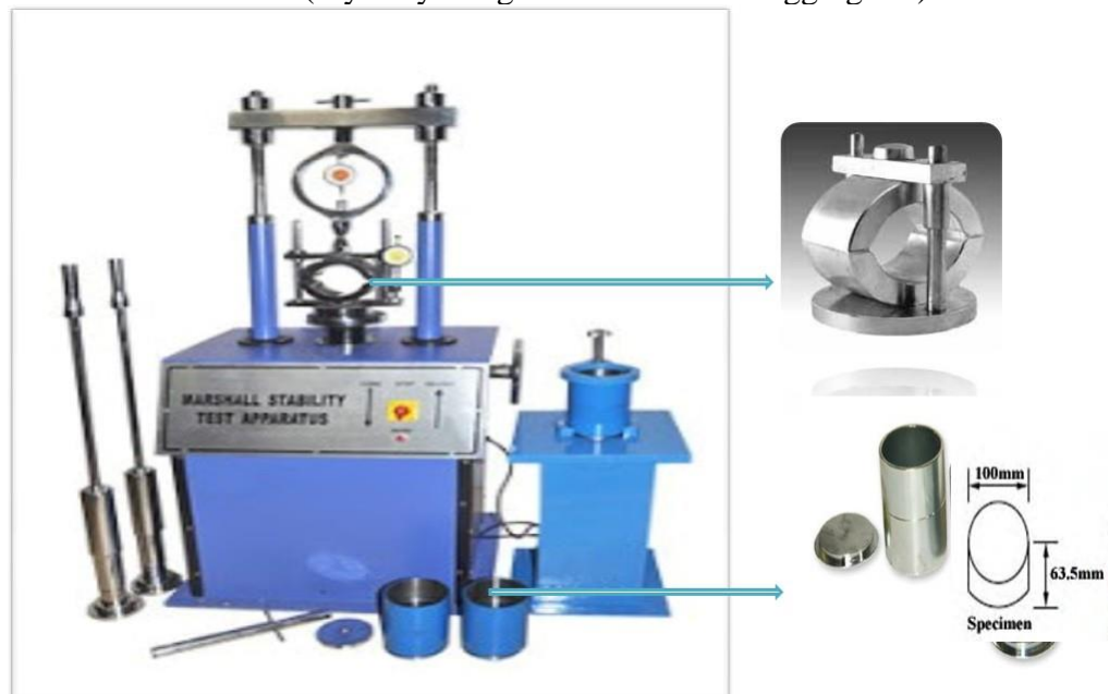
Figure 1. Marshall Stability Test
