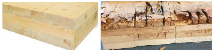
Figure 2. CLT and example of deterioration of CLT flooring under the influence of moisture (Kesik & Martin, 2021)
